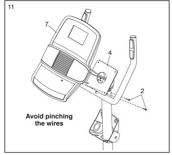
12. Slide the Console Cover (3) upward to the Handlebar (4). Attach the Console Cover to the Handlebar and to the Console (7) with two M4 x 16mm Screws (2).
