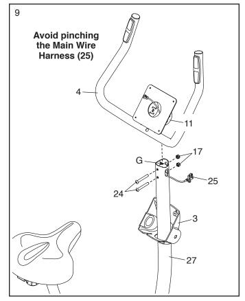
10. Untie and discard the wire tie on the Main Wire Harness (25). Route the Main Wire Harness upward through the Handlebar (4) as shown.
