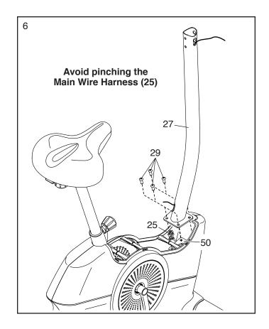
Locate the lower end of the wire tie (E) in the Upright (27). Tie the wire tie to the Main Wire Harness (25). Then, pull the upper end of the wire tie until the Main Wire Harness is routed through the Upright and out of the indicated hole (F).
