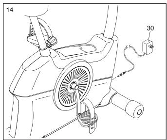
15. After the exercise bike is assembled, inspect it to make sure that it is assembled correctly and that it functions properly. Make sure that all parts are properly tightened before you use the exercise bike. Extra parts may be included. Place a mat under the exercise bike to protect the floor or carpet.
