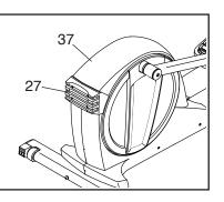
shown) from the Top Shield (37), and use a standard screwdriver to pry the Top Shield upward off the elliptical. Then, look into the access opening and locate the Reed Switch (58). Rotate the Pulley (66) until a Magnet (41) is aligned with the Reed Switch.
