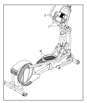
To dismount the elliptical, wait until the pedals (K) come to a complete stop. **Note: The elliptical does not have a free wheel; the pedals will continue to move until the flywheel stops.** When the pedals are stationary, step off the higher pedal first. Then, step off the lower pedal.
