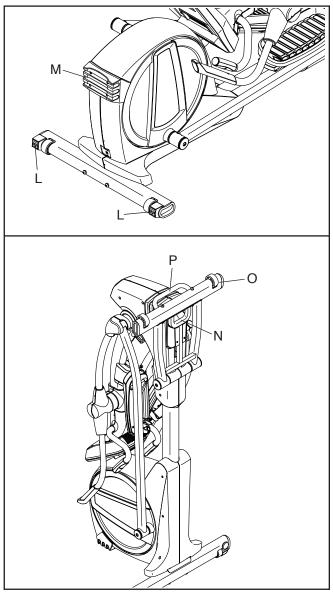
**See the lower drawing.** To lower the elliptical for use, first hold the handle on the lift frame (N) with one hand and hold the front stabilizer (O) with your other hand. Next, pull the frame toward you and lower it until you can reach the handle on the front stabilizer (P). Then, hold the handle on the front stabilizer with both hands and finish lowering the elliptical to the floor.
