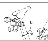
ment handle into an adjustment hole in the saddle post, and firmly tighten the adjustment handle three turns. Make sure that the adjustment handle is engaged in an adjustment hole. Then, pull the adjustment handle outward, turn it so that it points downward as shown, and then release it.
