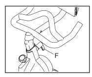
adjustment hole in the handlebar, and firmly tighten the adjustment handle three turns. Make sure that the adjustment handle is engaged in an adjustment hole. Then, pull the adjustment handle outward, turn it so that it points downward as shown, and then release it.
