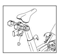
Note: The carriage handle (D) functions like a ratchet. Turn the carriage handle in the desired direction, pull it outward, turn it in the opposite direction, push it inward, and then turn it in the desired direction again. Repeat this process as many times as necessary.
