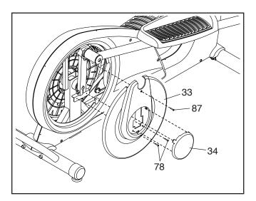
Then, remove the M4 x 16mm Machine Screw (87) and the two M4 x 16mm Screws (78) from the right Disc (33), and then remove the right Disc.
