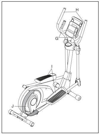
Push the pedals (I) until they begin to move with a continuous motion. Note: The pedal discs (J) can turn in either direction. It is recommended that you move the pedal discs in the direction shown by the arrow; however, for variety, you can turn the pedal discs in the opposite direction.
