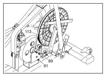
Reattach the right shield, the right roller arm, the right pedal arm, the shield cover cap, and the shield cover. Then, plug in the power cord.
