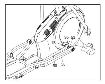
**See EXPLODED DRAWING C on page 43.** Identify the Left and Right Shields (73, 74). Remove the M4 x 19mm Screws (5) and the M4 x 48mm Screw (107) from the Left and Right Shields. Then, remove the Right Shield.
