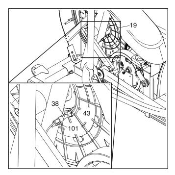
Loosen, but do not remove, the indicated M4 x 16mm Screw (101). Slide the Reed Switch (38) slightly closer to or away from the Magnet (43), and then retighten the Screw. Then, plug in the power cord, press the power switch to the reset position, and rock the Pulley (19) forward and backward just enough that the Magnet passes the Reed Switch repeatedly.
