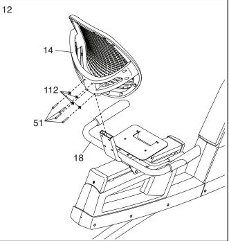
Attach the Seat (12) to the Seat Handlebar (18) with four M6 x 20mm Screws (67) and four M6 Washers (112) (only two of each are shown); start all the Screws, and then tighten them.
