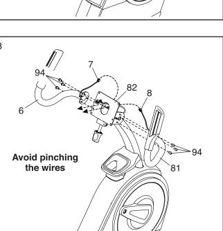
While a second person holds the Console (5) near the Console Bracket (82), plug the Main Wire (41) and the Left and Right Pulse Wires (7, 8) into the receptacles on the Console.
