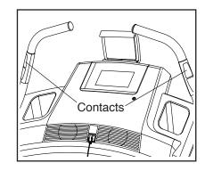
To measure your heart rate, stand on the foot rails and hold the contacts with your palms for approximately ten seconds; avoid moving your hands. When your pulse is detected, your heart rate will be shown. For the most accurate heart rate reading, continue to hold the contacts for about 15 seconds.
