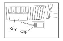
the key into the console. Note: It may take a minute for the console to be ready for use. IMPORTANT: In an emergency, the key can be pulled from the console, causing the walking belt to slow to a stop. Test the clip by carefully taking a few steps backward; if the key is not pulled from the console, adjust the position of the clip.
