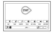
Manual button on the console, and then touch the Resume button on the screen. The walking belt will begin to move at 1 mph. As you exercise, change the speed of the walking belt as desired by pressing the Speed increase and decrease buttons. Each time you press one of the buttons, the speed setting will change by 0.1 mph; if you hold down the button, the speed setting will change in increments of 0.5 mph.
