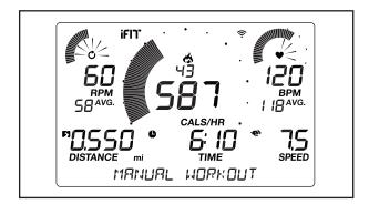
Calories (flame icon)—This display will show the approximate number of calories you have burned. When some onboard workouts are selected, this display will show the number of calories remaining to be burned for the workout.
