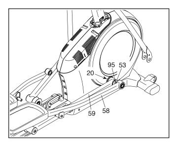
See EXPLODED DRAWING C on page 35. Identify the Left and Right Shields (73, 74). Remove the M4 x 19mm Screws (5), the M4 x 25mm Screws (127), and the M4 x 45mm Screw (107) from the Left and Right Shields. Then, remove the Right Shield.
