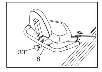
adjustment hole; make sure that the Seat Frame Pin is securely engaged.
