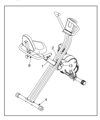
Next, pull upward on the Seat Frame (8) and pull the Frame Pin (13) outward with your other hand. Then, move the Upright (2) upward or downward until the exercise bike is in the upright position, and release the Frame Pin into the hole in the Frame (1); make sure that the Frame Pin is securely engaged in the Frame.
