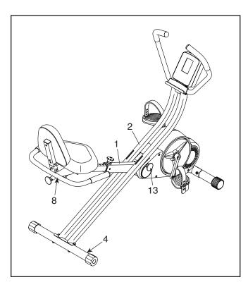
Next, pull upward on the Seat Frame (8) and pull the Frame Pin (13) outward with your other hand. Then, move the Upright (2) upward or downward until the exercise bike is in the recumbent position, and release the Frame Pin into the hole in the Frame (1); make sure that the Frame Pin is securely engaged in the Frame.
