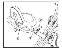
are in the lowest position. Hold the Seat Frame (8) in the indicated location. Then, loosen and pull the Seat Post Knob (31) outward, move the Seat Post upward or downward to the desired position, release the Seat Post Knob into an adjustment hole in the Seat Post, and then tighten the Seat Post Knob. Make sure that the Seat Post Knob is securely engaged in an adjustment hole.
