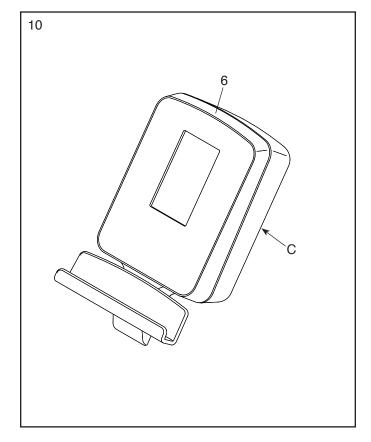
11. Have a second person hold the Console (6) near the Handlebar (5). Connect the Main Wire (87) to the receptacle on the back of the Console.
