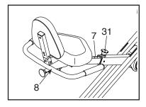
when the pedals are in the most forward position. Hold the Seat Frame (8) in the indicated location. Then, loosen and pull the Seat Post Knob (31) outward, move the Seat Post (7) upward or downward to the desired position, release the Seat Post Knob into an adjustment hole in the Seat Post, and then tighten the Seat Post Knob. Make sure that the Seat Post Knob is securely engaged in an adjustment hole.
