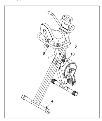
See the drawing at the left. Next, pull upward on the Seat Frame (8) and pull the Frame Pin (13) outward with your other hand. Then, move the Upright (2) upward or downward until the exercise bike is in the storage position, and release the Frame Pin into the hole in the Frame (1); make sure that the Frame Pin is securely engaged in the Frame.
