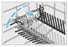
Upper rack flip tines: To fold down, push flip tines downward with gentle pressure. To fold up, push flip tines into an upright position until the holder engages in the notch.
