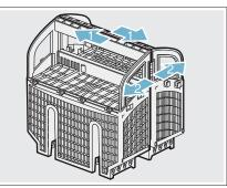
To assemble the Double Flex silverware basket: Hold the two halves side by side or back to back, so that the tab on one basket can slip into the notch on the other basket. Push the two halves in opposite directions until they click. **Note:** The silverware basket lid may also be folded downward in order to leave the basket open.
