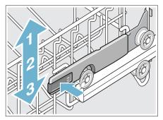
**Note:** Check spray arm for clearance after adjustment.
