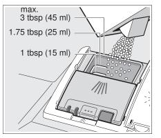
When using detergent tabs, lay them such that they do not come in contact with the cover, insert a detergent tab flat, not on its side. **Note:** Do not place detergent tabs or utensils in the detergent tab tray 24. Place tabs or other detergent forms directly in the detergent dispenser 32.
