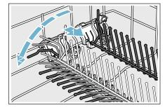
Upper rack flip tines: To fold down, push flip tines downward with gentle pressure. To fold up, push flip tines into an upright position until the holder engages in the notch.
