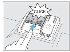
The detergent dispenser will open automatically at the ideal time for the set cycle. The powder or liquid detergent is distributed in the appliance and is dissolved, detergent tabs will fall into the detergent tab tray 24 where it dissolves during the cycle.
