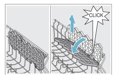
Removing/Installing third rack
