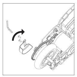
1. Using a 4mm hex wrench remove the 2 bolts from the rear chain cover on side of the scooter
