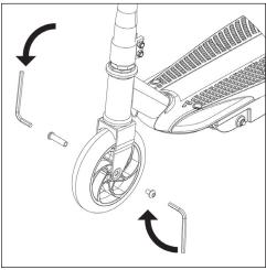
3. Reinstall hardware and tighten clockwise with a 5mm hex wrench.
