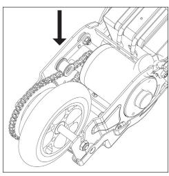
5. Place the chain under tensioner wheel and onto the rear chain wheel gear and install replacement wheel into the frame. Do not tighten axle nuts yet.
