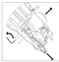
4. If replacing the chain, remove the motor bolts with a 4mm hex wrench. Slide motor out of the frame slightly so that there is enough room to remove/replace the chain onto the motor gear. Replace spacers and retighten bolts.
