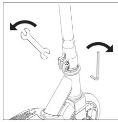
2. Tighten the bolts with the 5mm hex wrench and 10 mm wrench. Tighten bolts evenly and securely.
