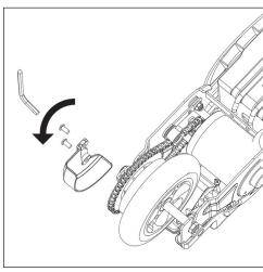
7. Reinstall chain cover with a 4mm hex wrench. Do not over tighten bolts.
