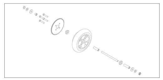
3. Note the location of all rear wheel hardware and ensure to properly reinstall all items.
