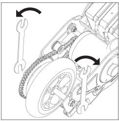
6. Ensure axle washers are seated correctly against the frame. After tightening axle nuts with 13mm wrenchs check wheel alignment and the tracking of the chain by rotating the wheel counter clockwise with your hand. Wheel should spin freely and easily.
