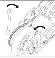
2. Using two 13mm wrenches loosen the rear wheel axle nuts. Pull up on the chain tensioner and remove the rear wheel from the frame.
