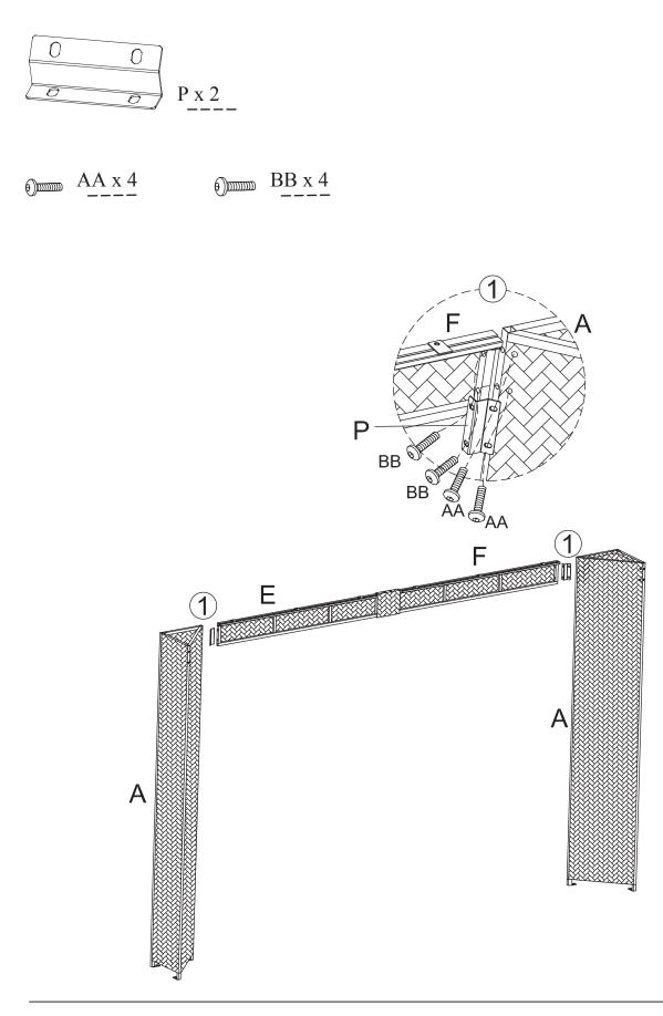
**6.** Secure long crossbar and Post (A) with fixed plate (P) by Bolt (AA, BB) (see figure 1). Fully tighten once all bolts on position.
