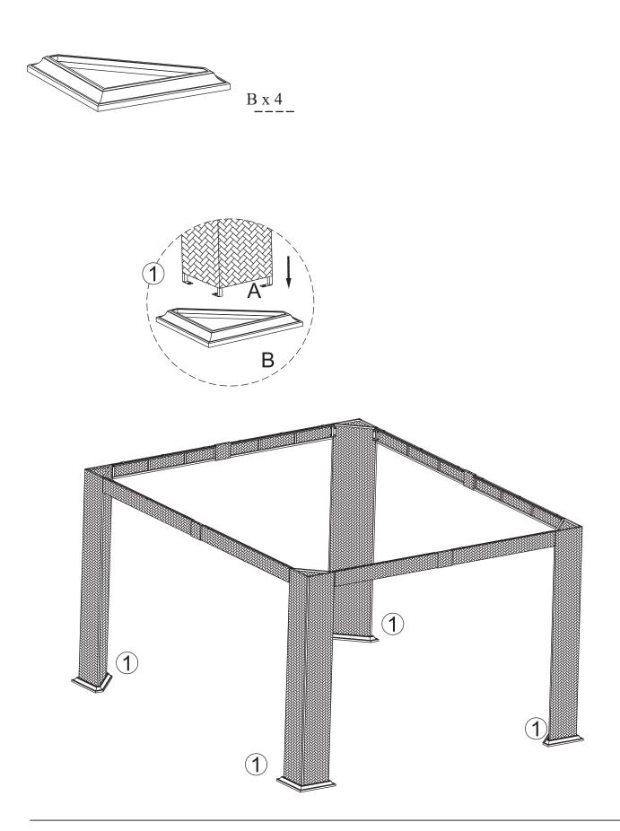
**8.** Insert Roof tube (K) into Corner roof tube (L). Insert another side of Roof tube (K) into Roof connector (J) (see figure 2) then secure another side of Corner roof tube on the top of Post (A) with Bolt (AA).
