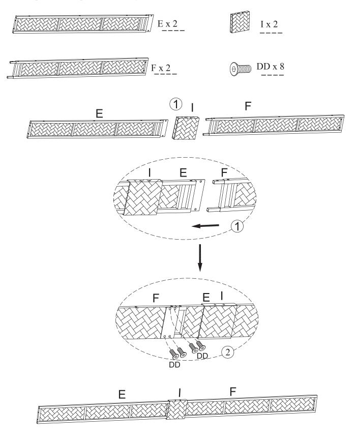
2. Insert Center connector (I) into Long crossbar (H), then insert Long crossbar (G) into Long crossbar (H) as figure 1 shown. Secure Long crossbar (H) with Long crossbar (G) using Bolt (DD) as figure 2 shown. Then move Center connector (I) to the center of short crossbar.
