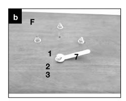
3. Attach connector panel (F) to the post (B) using four nuts (1), four spring washers (2) and four large flat washers (3) as shown in inset (b). Tighten the nut with the open-end wrench (7).
