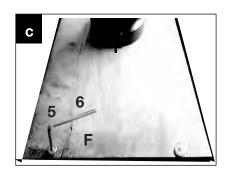
4. Attach the connector panel (F) to the supports (D&E) using four short Allen bolts (5), as shown in inset (c). Tighten the bolts with an Allen wrench (6).
