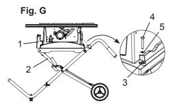
**NOTE:** Before using the saw, verify that the table saw is securely locked in position.
