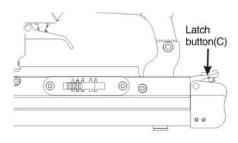
Insert a stick of fasteners into the magazine with pins positioned as shown, make sure pins are not dirty or damaged. Pins are marked for direction of loading.
