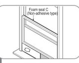
Cut the non-adhesive foam seal C to match the width of the window. Insert the seal between the glass and the window frame to prevent air and insect from getting into the room.
