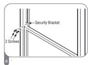
If desired, install the security bracket with 2 screws.
