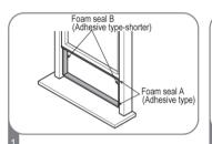
Cut the adhesive foam seal A and B strips to the proper lengths and attach them to the window sash and frame
