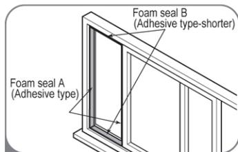
1 Cut the adhesive foam seal A and B strips to the proper lengths and attach them to the window sash and frame.
