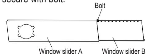
Note: If the window opening is less than the minimum length of the slider kit, cut Slider A. Cut the solid end, DO NOT cut out the openings.
