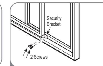
4 If desired, install the security bracket with 2 screws.
