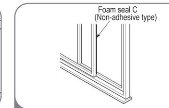
3 Cut the non-adhesive foam seal C to match the length of the window. Insert the seal between the glass and the window frame to prevent air and insect from getting into the room.
