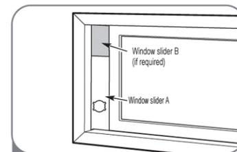
2 Insert the slider kit assembly into window opening.
