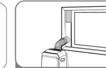
5 Insert the slider kit adaptors into the holes on the slider kit.
