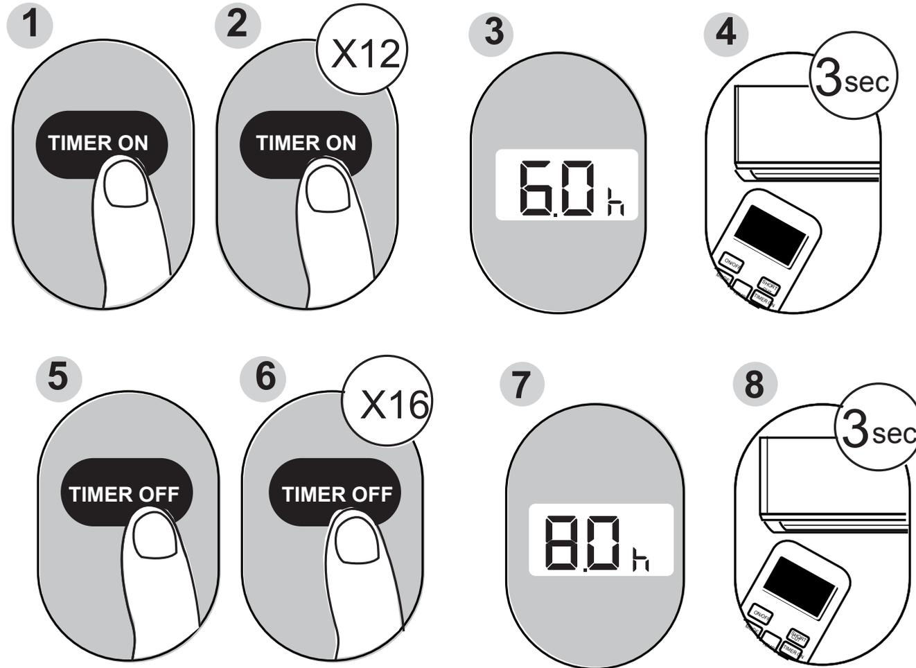
**Example:** Setting the unit to turn on after 6 hours, operate for 2 hours, then turn off (see the figure below).
