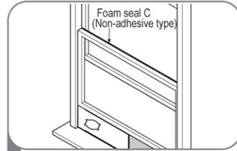
3 Cut the non-adhesive foam seal C to match the width of the window. Insert the seal between the glass and the window frame to prevent air and insect from getting into the room.
