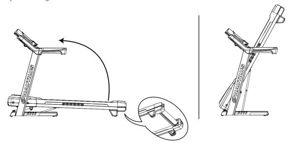
5. Make sure that the locking mechanism is engaged. Carefully pull back on the walking deck and make sure that it does not move. When you do this, keep clear of movement path in case the treadmill lock is not engaged.
