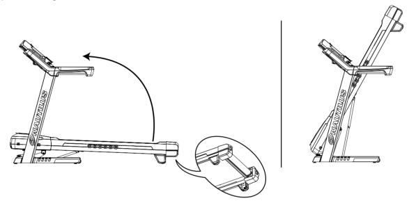
4. Make sure that the locking mechanism is engaged. Carefully pull back on the walking deck and make sure that it does not move. When you do this, keep clear of movement path in case the treadmill lock is not engaged.
