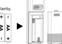
**Step 2:** Insert 2 *new* AA Alkaline batteries (not included) into the station. Observe the correct polarity.
