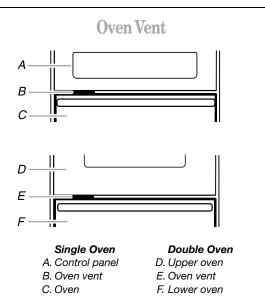
The oven vent should not be blocked or covered since it allows the release of hot air and moisture from the oven. Blocking or covering vents will cause poor air circulation, affecting cooking and cleaning results. Do not set plastics, paper or other items that could melt or burn near the oven vent.
