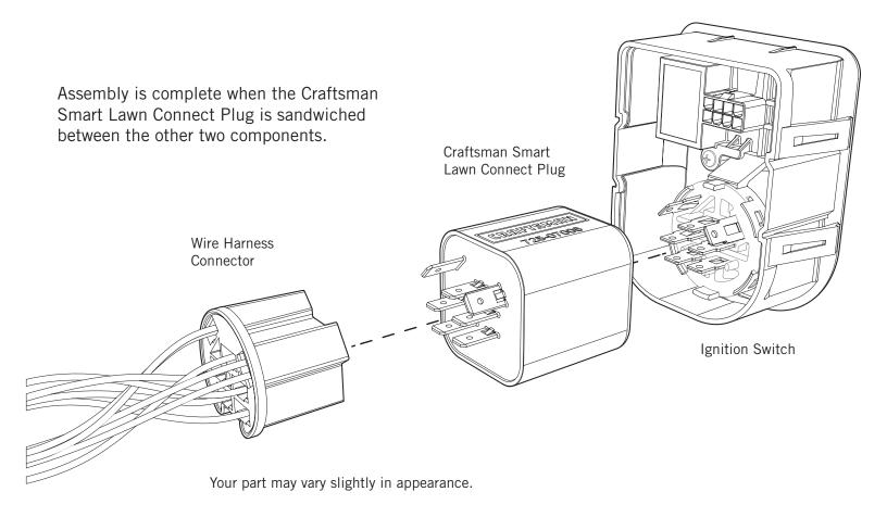
4 When all three components are plugged together this is how the plug assembly looks (refer to illustration below). NOTE: The base of the **Ignition Switch** prongs will be visible in the gap between the **Ignition Switch** and the **Craftsman Smart Lawn Connect Plug**. This is intentional, and allows for proper plug functionality.
