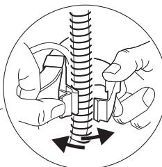
The drain hose is secured in place with two plastic latching clamps. Press the locking tab and release the drain hose.
