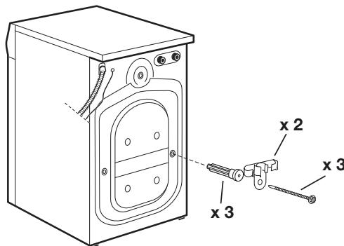
Remove all of the following from the back of the washer:
