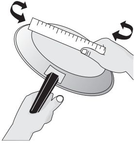
Figure 1: Check pan for flat bottom using ruler
