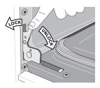
Figure 22: Hinge lock/unlock positions
