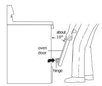
Figure 23: How to remove door
