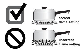
Figure 8: Correct and incorrect flame settings
