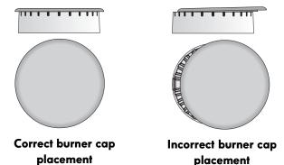
Figure 4: Burner cap placement
