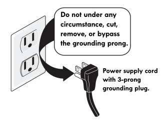
Figure 1: Grounding type wall receptacle
