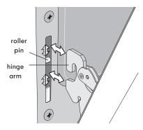
Figure 24: Hinge pin locations
