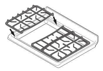
Figure 6: Burner grates placement
