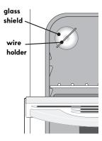
Figure 20: Replacing the oven light
