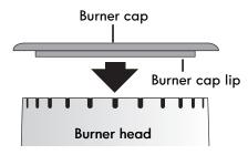
Figure 3: Burner cap lip placement
