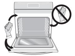
Figure 15: Clean around the oven door gasket
