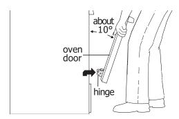
Figure 22: Holding door for removal
