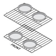
Figure 11: Pan positions two rack baking
