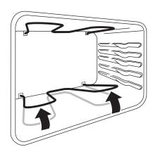
Figure 19: Lift bake element
