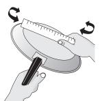
Check for flatness by rotating a ruler across the bottom of the cookware (see Figure 1). Cookware should have flat bottoms that make good contact with the entire surface heating element (see Figure 2).
