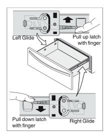
Figure 25: Parts of storage drawer
