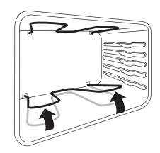
Figure 8: Lift bake element
