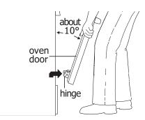
Figure 11: Holding door for removal
