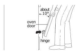
Figure 14: Holding door for removal
