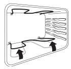
Figure 10: Lift bake element
