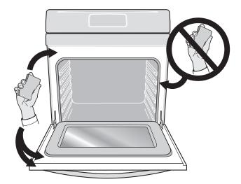
Figure 8: Oven door area to clean and not clean (gasket).
