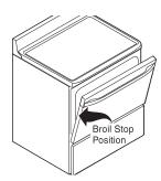
Figure 5: Door open for broiling
