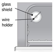
Figure 4: Oven light protected by glass shield
