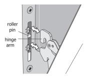
Figure 10: Replacement and location of hinge arm and roller pin
