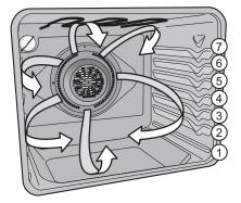
Figure 3: Air movement using convection
