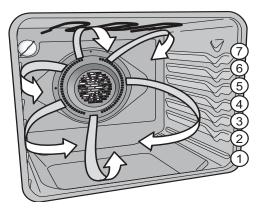
Figure 8: Convection fan circulation
