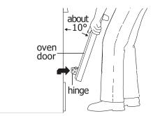
Figure 9: Holding door for removal
