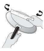
Check for flatness by rotating a ruler across the bottom of the cookware (see Figure 1). Cookware should have flat bottoms that make good contact with the entire surface heating element (see Figure 2).
