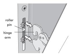
Figure 32: Hinge pin locations
