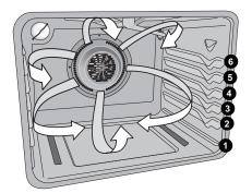
Figure 18: Air movement using convection
