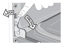
Figure 30: Hinge lock/unlock positions
