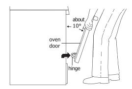
Figure 31: How to remove door
