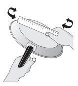
For best cooking results, cookware should have flat bottoms that rest level on the surface burner grate. Before using cookware, check for flatness by rotating a ruler across the bottom of the cookware (See Figure 5).
