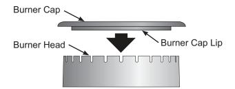
For proper gas flow it may be necessary to clean the burner head and slots. To clean, first use a clean DAMP cloth to soak up any spills. Remove any food from between the burner slots using a small nonabrasive brush like a toothbrush and afterwards wipe up using a damp cloth. For stubborn soils located in the slots, use a small-gauge wire or needle to clean.
