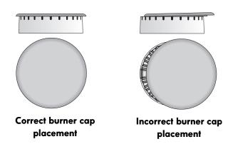
Figure 2: Burner cap placement
