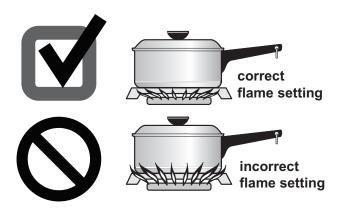
Figure 6: Correct and incorrect flame settings
