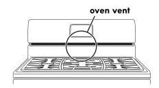
Figure 8: Do not block oven vent location
