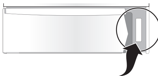
Figure 2: Serial plate location
