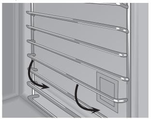
Insert the two lower prongs of the support into the two lower holes in the cavity wall, as show below. Push down the oven rack support into its resting position.
