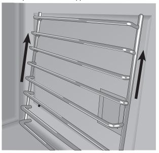
Tilt the lower part of the rack support toward the cavity wall, as shown below.
