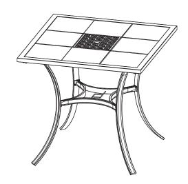
• Tighten all bolts in a diagonal pattern.
