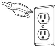
Washer must be electrically grounded in accordance with local codes and ordinances, or in the absence of local codes, in accordance with the NATIONAL ELECTRICAL CODE, ANSI/NFPA NO. 70 latest edition. Check with a licensed electrician if you are not sure that the washer is properly grounded.
