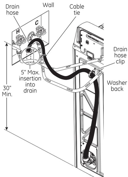
**NOTE:** Placing the drain hose too far down the drain pipe can cause a siphoning action. No more than 5" of hose should be in the drain pipe. There must be an air gap around the drain hose. A snug fit can also cause a siphoning action.
