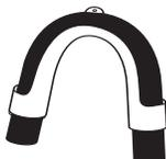
**NOTE:** Install hose guide on hose end if equipped.
