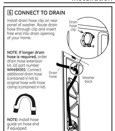
**If water valves and drain are built into wall,** fasten drain hose to one of the water hoses with cable tie provided.
