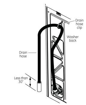
**NOTE:** Placing the drain hose too far down the drain pipe can cause a siphoning action. No more than 5" of hose should be in the drain pipe. There must be an air gap around the drain hose. A snug fit can also cause a siphoning action.
