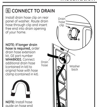
**If water valves and drain are built into wall,** fasten drain hose to one of the water hoses with cable tie provided.
