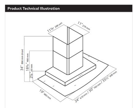
**Note:** The vent hood must be installed 24" min., and 36" max. above the cooking surface.
