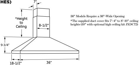
The vent hood must be installed 24" min. and 36" max. above the cooking surface. The hood installation height above the cooking surface depends upon ceiling height. The telescopic duct cover conceals the ductwork running from the top of the hood to the ceiling.
