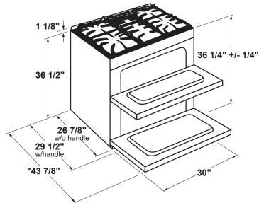
\*Dimensions are referenced from the point at the back of the range that will contact the rear wall first.
