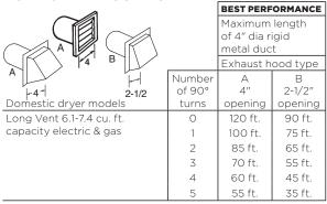
For every extra  $90^{\circ}$  elbow, reduce the allowable vent system length by 10 ft.
