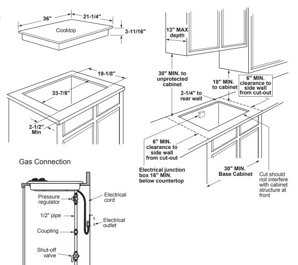
Dimension and installation information are shown in inches. \*Allow 5-3/4" depth at rear for electrical and gas connections
