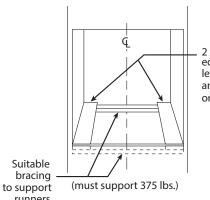
equivalent runners level with bottom of cutout and flush with sides of cutout or solid bottom floor.
