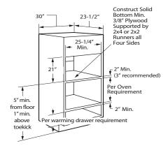
\* For existing cutouts, a maximum width of 28-1/2" is acceptable. If the opening is slightly wider, secure a furring strip on each side of the cutout for securing the oven.
