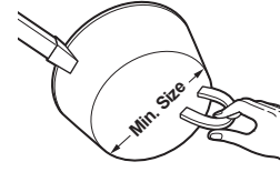
Use the minimum size pan for the element. The pan material is correct if a magnet sticks to the bottom.
