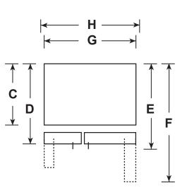
$\mbox{^\dagger} Water$  hook-up fits in back air clearance when calculating installation depth.
