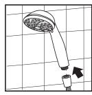
Put washer into nut on other end of hose and hand tighten nut to hand shower.
