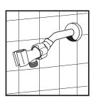
3. Insert screen washer into mounting bracket and hand tighten onto shower arm. Do not overtighten.
