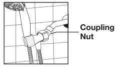
6. Fit hand shower into mounting bracket by slipping the hose through the bracket opening and seating the hand shower into the bracket. Loosen coupling nut and adjust the position of the hand shower as needed.
