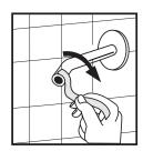
2. Apply 2 revolutions of thread tape to threads of shower arm. Make sure the tape is applied tightly in a clockwise direction.
