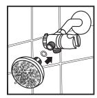
4. With washer positioned in showerhead, hand tighten showerhead to diverter bracket.
