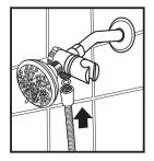
5. Place washer into one of the hose nuts and hand tighten to diverter bracket.
