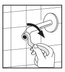
2. Apply 2 revolutions of thread tape to threads of shower arm. Make sure the tape is applied tightly in a clockwise direction.
