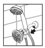
7. Place handheld shower into bracket by slipping the hose through the bracket opening and seating the shower into the bracket. If the bracket does not maintain its position when the handheld is placed into the bracket, reposition bracket and wrench tighten another 1/4 turn.
