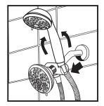
8. To adjust position of the handheld shower, push the handheld shower back or pull it forward while you hold the diverter bracket.
