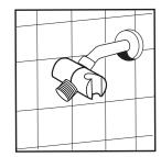
3. With screen washer preassembled in diverter bracket, hand tighten diverter bracket to shower arm. Position diverter bracket as shown in picture and then wrench tighten 1/4 turn. Do not over tighten.
