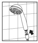
6. Put washer into nut on other end of hose and hand tighten to handheld shower.
