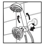
8. To adjust position of the handheld shower, push the handheld shower back or pull it forward while you hold the diverter bracket.
