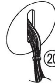
Use enclosed wire management clip to keep the wires together.
