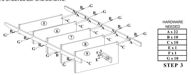
3. USING PICTURE AS A GUIDE, ATTACH SMALLEST SHELF (5) TO TOP OF RAIL, USING 2 WOOD DOWELS (A) AND 1 BOLT (B). REPEAT THIS PROCESS FOR ALL SHELVES BEFORE ATTACHING SECOND RAIL TO UNIT. USING 2 DOWELS AND 1 CAMLOCK/BOLT, FASTEN BOTTOM LEG TO LARGEST SHELF.
